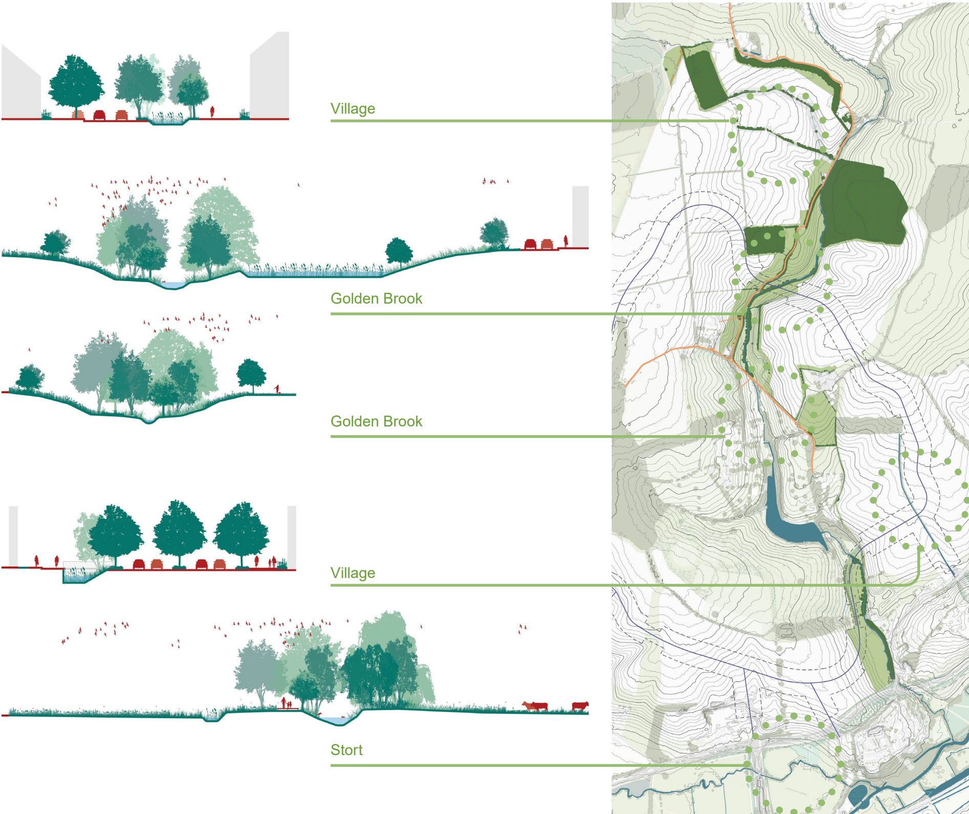
Fig.154 Illustrative sections exploring various SuDS feature characters along Golden Brook and Fiddler's Brook Valleys
